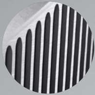
Laser engraving Surface finish reduced to Ra 1.0 µm
